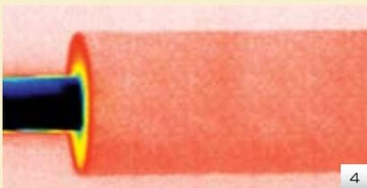
**Fig. 4** Infrared photo shows thermal energy emitted from the fiberglass insulated on low temperature pipe before water absorption test, which shows good thermal insulation performance of dry fiberglass insulation.
