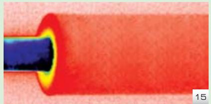
**Fig. 15** Infrared photo shows thermal energy emitted from Aeroflex insulated on low temperature pipe after 20 minutes of water absorption test, [ASTM D 1056 water absorption approx. 4% by weight] which shows good thermal insulation performance.
