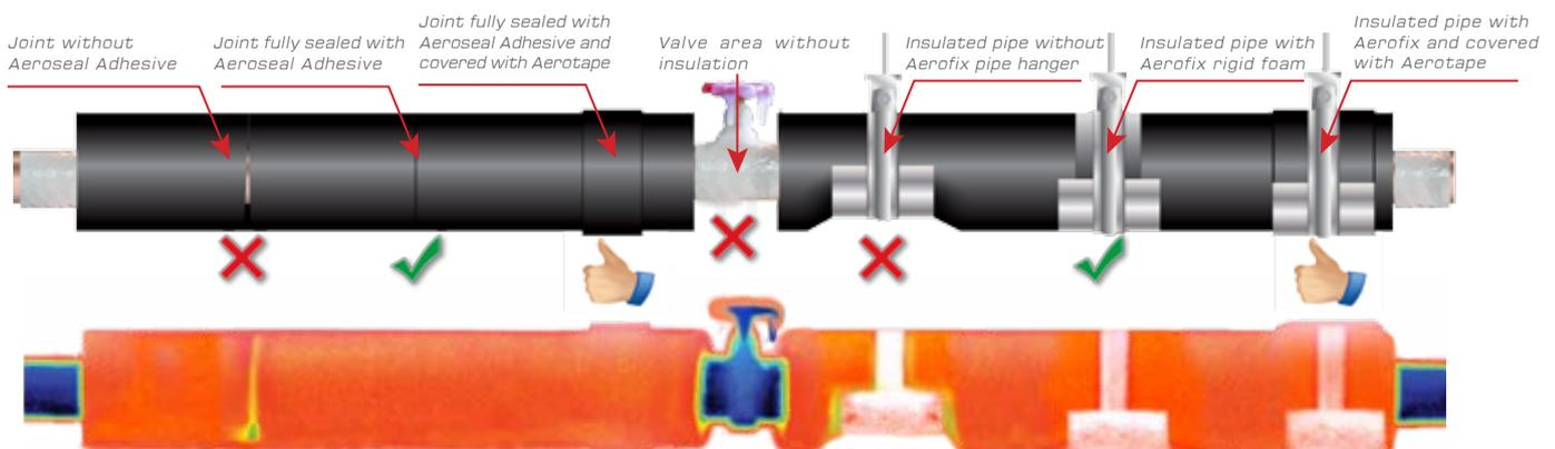
Fig.5 The illustration shows the do and don't when installing Aeroflex insulation on low temperature pipeline to prevent condensation.
