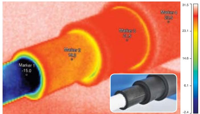
Infrared photo shows thermal emission from low temperature pipe without and with various thickness of Aeroflex thermal insulation. If surface temperature of insulation below dew point, condensation occurs.
