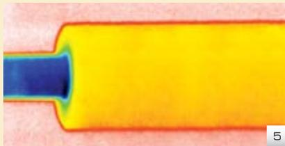
**Fig. 5** Infrared photo shows thermal energy emitted from the fiberglass insulated on low temperature pipe after 20 minutes of water absorption test, [ASTM D 1056 water absorption approx. 400% by weight] which shows poor thermal insulation performance of wet fiberglass insulation.
