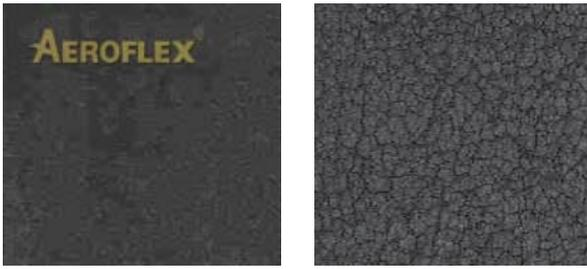
**AEROFLEX - EPDM (NON CRACK) OTHERS - NBR/PVC (CRACK)**
