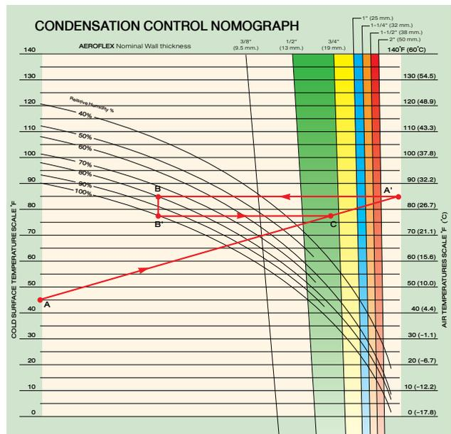
Fig.1 Condensation Control Nomograph is a convenient tool for determining insulation thickness to prevent condensation.
