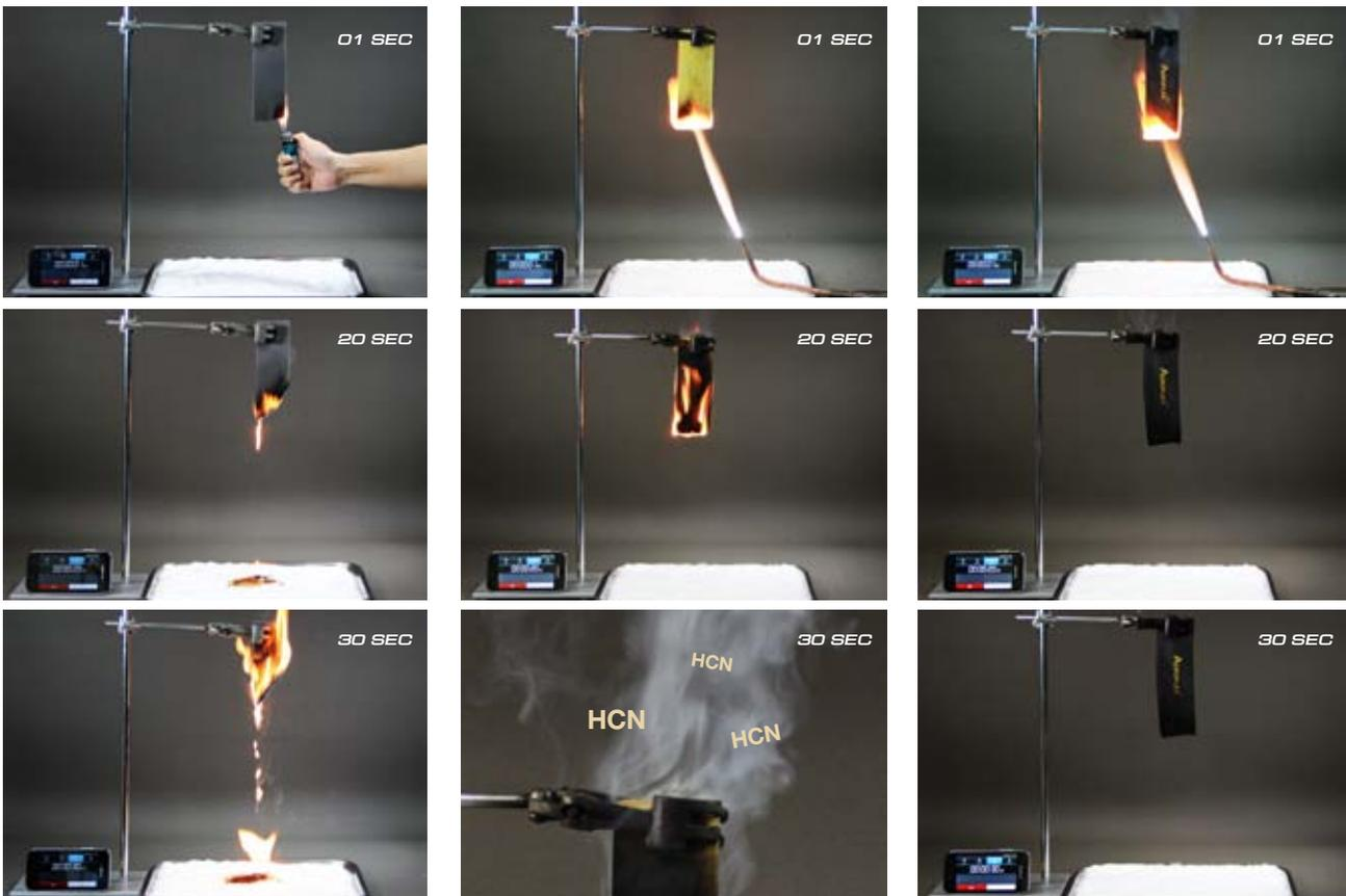
**PE. Foam :** this plastic insulation is manufactured from polyethylene plastic with tiny cells containing butane or similar gases, making the density approx. 2 lb/ft<sup>3</sup>. Most PE Foam insulation is highly combustible and can cause rapid flame transfer. It will melt and generate flaming balls (fire balls), causing flame transfer to other materials in buildings such as ceilings, carpets, and furniture.
