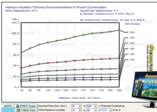
Fig.2 Minimum insulation thickness recommendation graph and data table shows Aeroflex insulation thickness required to prevent condensation at various %RH and various pipe sizes. Aeroflex calculation program also calculates energy loss & gain, economic thickness and other calculation for HVAC&R industry.
