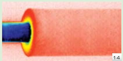
**Fig. 14** Infrared photo shows thermal energy emitted from Aeroflex insulated on low temperature pipe before water absorption test, which shows very good thermal insulation performance of dry Aeroflex insulation.
