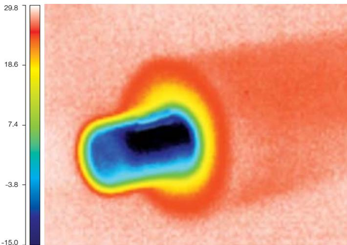
Infrared photo shows thermal energy emitted from refrigeration piping with appropriate thickness of thermal insulation for energy-saving and preventing condensation [see more details on page 18, 19 and 20 "Condensation Control" and "Recommendation"]
