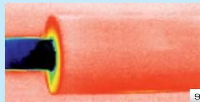
**Fig. 9** Infrared photo shows thermal energy emitted from PU foam [45 kg/m<sup>3</sup>] insulated on low temperature pipe before water absorption test, which shows a very good insulation performance of dry PU foam insulation.
