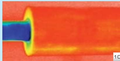
**Fig. 10** Infrared photo shows thermal energy emitted from PU foam [45 kg/m<sup>3</sup>] insulated on low temperature pipe after 20 minutes of water absorption test, [by ASTM D 1056, water absorption is approx. 40% by weight] which shows fair thermal insulation performance.
