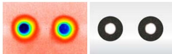
Fig.4 Infrared photo shows thermal energy around insulated pipes located 4" apart, allowing free air movement without accumulation of moisture and no condensation problem.
