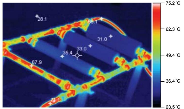
*Infrared photo shows thermal energy emitted from hot water piping without thermal insulation and with various thickness of insulation, illustrating less thermal energy emittance from thicker insulation.*
