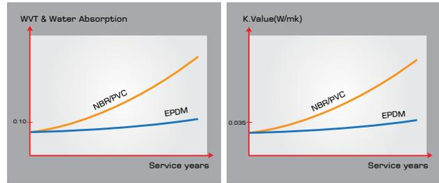
Low water vapor transmission, low water absorption and durability of material are very important factors for maintaining insulation properties during service, especially used in cooling system, EPDM based insulation has excellent durability, so Aeroflex is more stable in thermal conductivity [K value], less water absorption and less moisture penetration than other insulations that are made of NBR/PVC.
