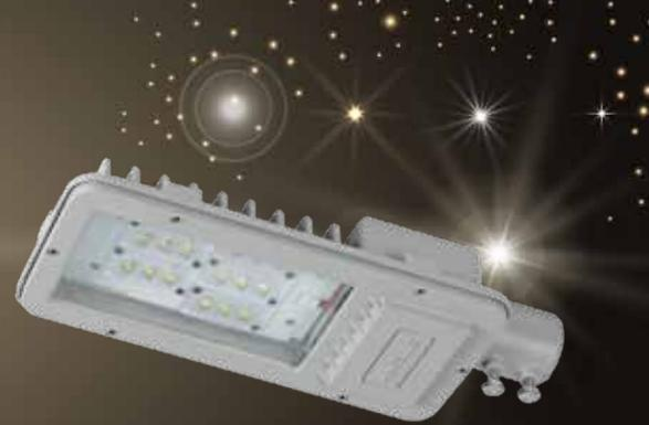
LED streetlight made up of pressure die cast housing with toughened glass and individual high power LEDs with secondary optics, IP66 protection, impact resistance of IK07 & 10 KV external SPD.
