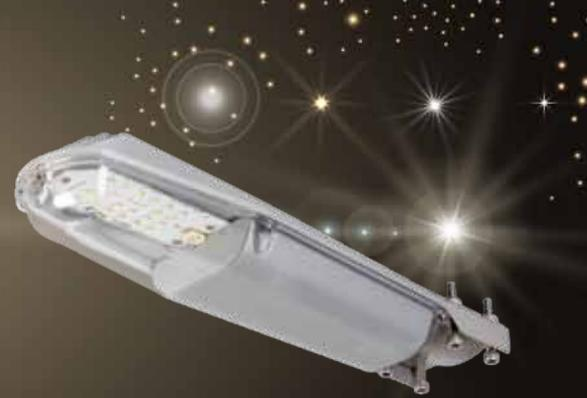
Energy saving and environmental friendly long life LED street light made up of pressure die cast aluminium housing with acrylic cover as diffuser with IP66 protection and Impact resistance of IK07.
