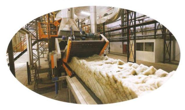
The factory utilizes highly advanced technology to melt basalt at 1400°C to make the flowing lava spin at high speed using the latest multi spun disc system to produce hairline fibers which are bound together by spraying with a heat setting resin. The fibers are spread in a conveyor using the pendulum method to achieve an even distribution of density throughout the surface of the resulting products. A special additive is impregnated to the bonded material to make it water resistant.
