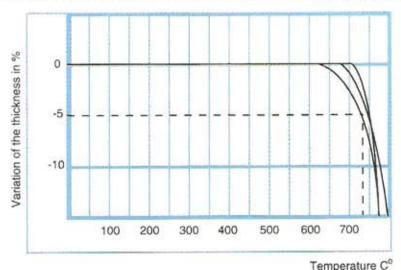
As tested in accordance with DIN 52271, Fujairah Rockwool products can be used at continuous working temperature up to 780°C without losing any of its insulating properties. Figures are shown above.
