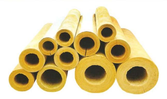
Fujairah Rockwool Preformed Pipe section conforming to ASTM C-547 and equivalent BS 3958-4 is intended for the thermo-acoustic insulation and fire protection of pipe works operating at high temperatures.
