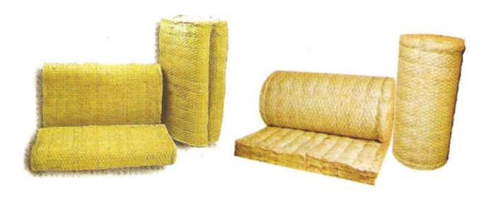
Fujairah Rockwool Blanket conforming to ASTM C-592 and equivalent BS 3958 Part 3 is a lightly bonded insulating material faced with hexagonal G.I. or S.S. wire mesh on one or both sides to form a firm but flexible multi-purpose insulating materials.
