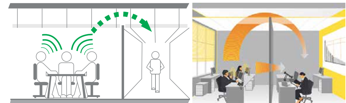
Room to room sound transmission through the ceiling
