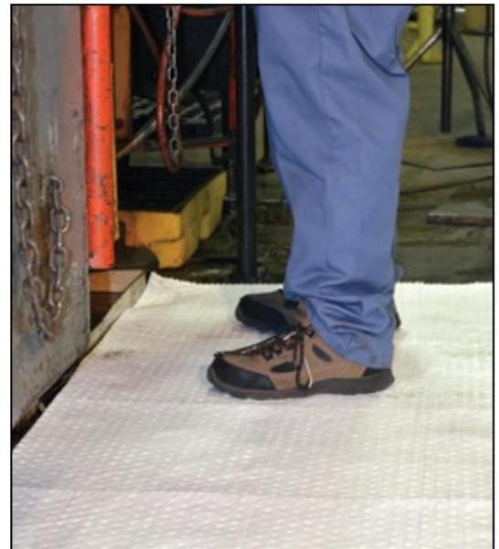
Use sorbent rolls to clean up workstation floors and reduce potential accidents.
