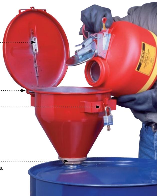
Fusible link melts at 165°F (74°C) and cover snaps shut to extinguish flames.
